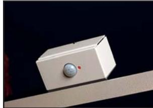
The motion sensor defaults to 20% light level, but it can be set at 0% (off) or 50%. The sensor can be easily turned off to keep the lights on. When using the sensor, it will dim the lights after no motion is detected in the aisle for 30 seconds. Once motion is detected, the lights will ramp up to 100% in just over a second.
